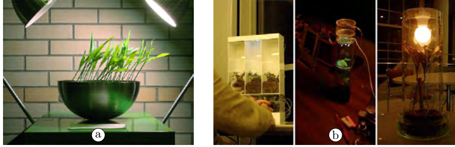
Fig.18: Examples of plant-based physicalization. (a) Infotropism is a robotic plant that grows into the direction of one of two lamps, which turn on depending on the use of a recycling bin [59]. (b) PlantDisplay treats growth of plants as a way of information display, by connecting the watering and the lighting of the plant to data sources [87].
