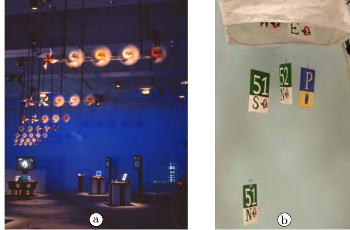
Fig.17: Examples of early ambient displays. (a) The Pinwheels installation presents information within a space through subtle changes in light, sound, and movement, which can be processed in the background of awareness [68,174]. (b) The BusMobile installation indicated how close each used bus was to the nearest bus stop by changing the height of the corresponding bus number [98].
