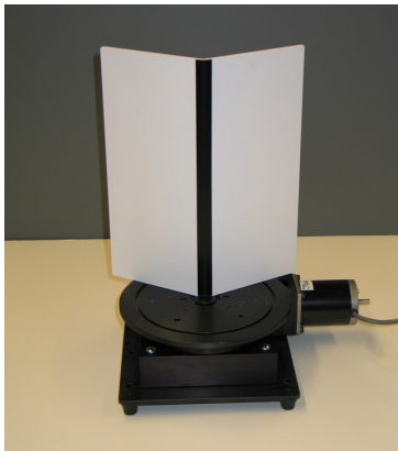
Fig. 4. Computer-controlled turntable and calibration chart used in laser scanning.
