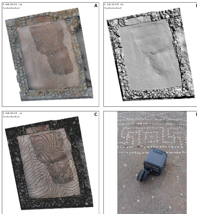
Fig. 1. Orthophoto (A) showing N-S17-2 mosaic. Shaded relief (B) and contour map (C) images of the topographical model extrated from the orthophoto. Proceq GP8800 GPR system (D) used for this investigation.
