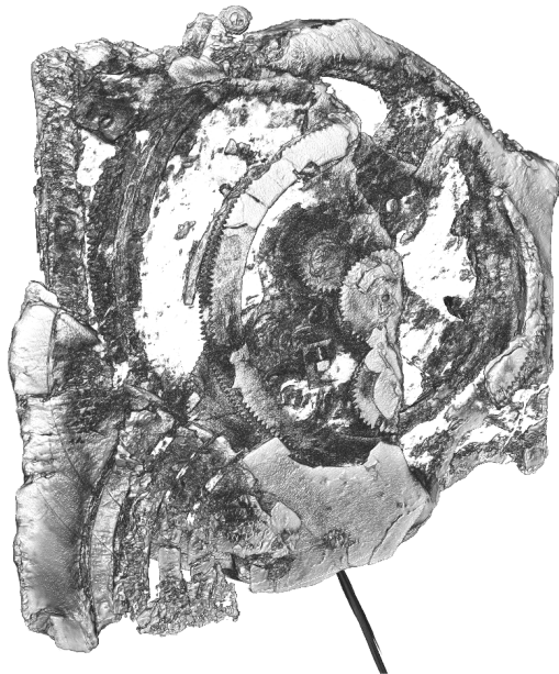
Figure 4. Tomography of fragment A of Antikythera Mechanism. This image is captured by the author in Computer and Network Systems Technology Laboratory (CNST-Lab), Department of Applied Informatics in University of Macedonia (Thessaloniki, Greece), using the "ImageVis3D" software package [9]
