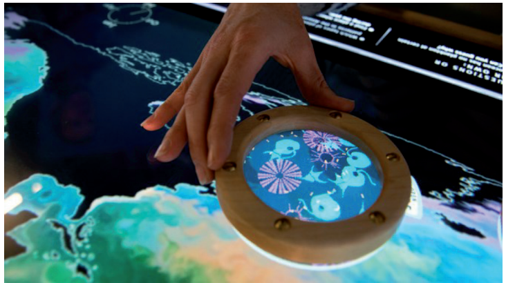
Figure 7. A close-up of one of the physical viewing lenses used as a tangible user interface to view the types of plankton species in various parts of the ocean. An infrared reflective fiducial marker engraved on the lens lets the table know its position and orientation. This is coupled with a virtual interface that moves under the physical lens and can provide more information about each species.
