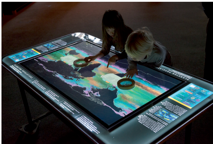
Figure 6. Museum visitors interacting with the plankton visualization. The custom-built table houses a Dell OptiPlex 990 and a 55-inch MultiTaction Cell. It's placed in an open area so that visitors can access and interact with the visualization from all sides. Labels placed around the table help guide and inform the viewer about exhibit content.
