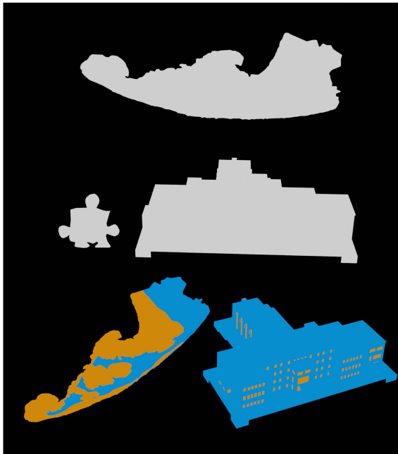
FIGURE 6. Silhouettes of our tracked models. Outer object silhouettes for Pauline Cove, Old Sun, and the platform are presented in white. Subobject silhouettes (occluded by the blue main objects, as in our tracking implementation) appear in orange.
