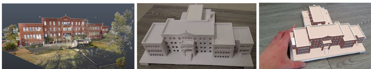
FIGURE 2. From left to right, the point cloud data, 3-D print, and AR overlay for Old Sun Community College.
