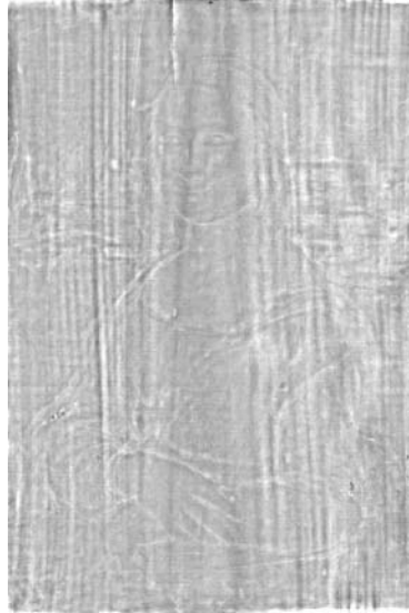
5 Local depth variations of the painting surface computed at a global scale. Wood grain and paint layer thickness variations are clearly visible.
