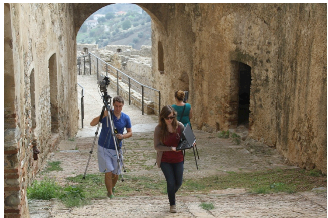
Figure. 2 - CISA3 Terrestrial Laser Scanning and Thermal Imaging teams utilizing specially adapted automated turrets digitally documenting Castello Svevo di Rocca Imperiale in southern Italy.
