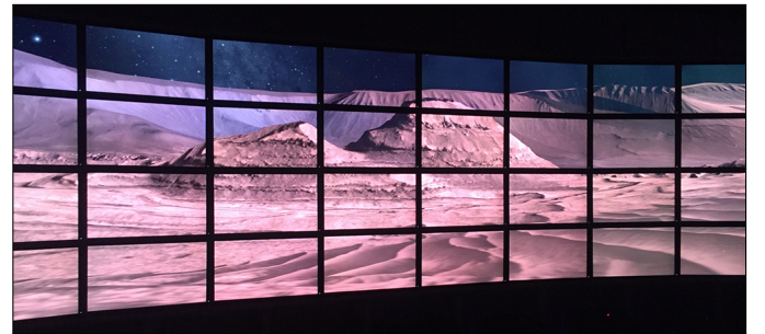
Fig. 6: Browsing the surface of Mars in a clustered environment rendering on the power wall at the University of Utah. The system uses eight rendering nodes, each connected to four screens.
