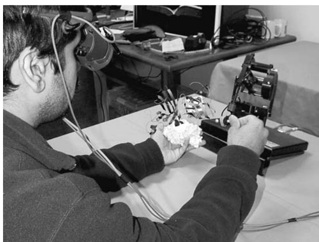
Fig. 8 User interacting with SOD model using a head-mounted display and aPHANTom haptic device. Virtual overlay shows SOD secondary structure and electrostatic force fields
