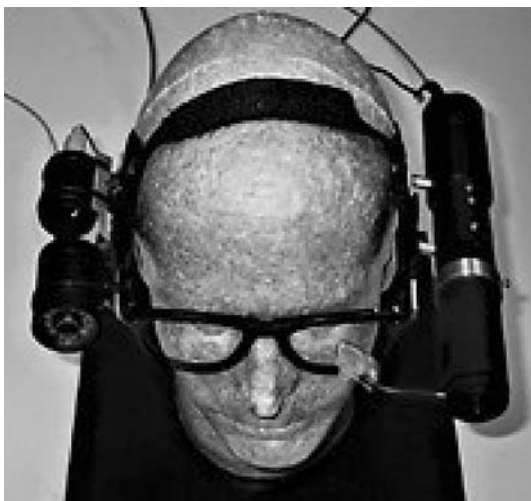
Fig. 2 A prototype wearable low vision aid, using head-mounted IR sensors and a scanned light display
