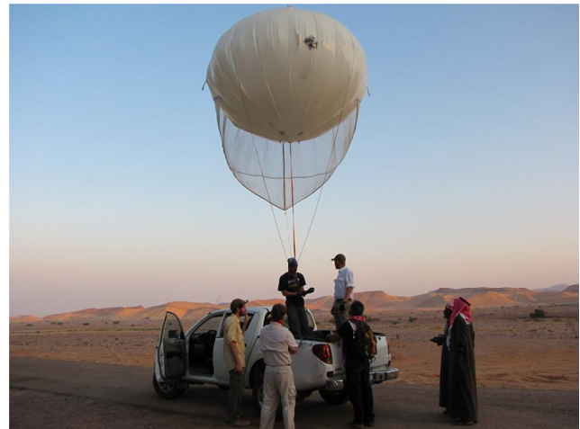
Fig. 3. The low altitude aerial balloon used for daily aerial SfM reconstructions. The balloon was inflated full during the entire season requiring only taping off every week the helium.
