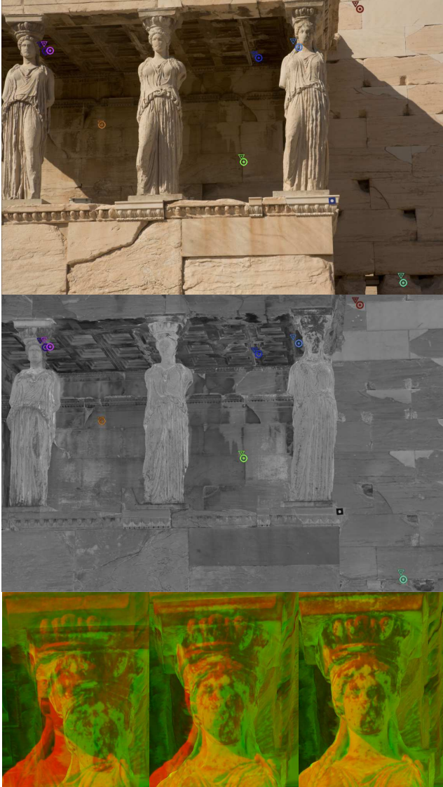
Fig. 1. A typical image of the Erechtheion: Distinct background and foreground causing big differences under pose rotation, strong cast shadows, significant differences in intensity. Top : 2D image (triangle SIFT points). Middle : 3D rendering (round SIFT points). Bottom : typical image difference for a small section after mouse (left), quick SIFT (middle), and image based (right) phases.
